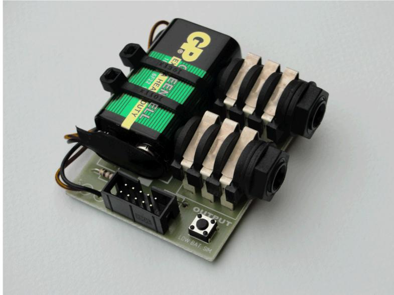
DBT module makes presentation of the sound of TM easy. While using DBT module there is no need to solder and install the preamp in a guitar. To link particular modules, just follow the instruction in the picture [the modules can be linked in any order]. Connect the DBT module output to amplifier input. Connect the guitar to the DBT input. While TM preamp presentation the guitar with passive output is recommended.
